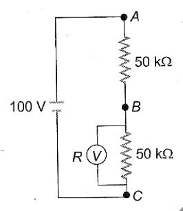
Internal resistance of voltmeter is R.
