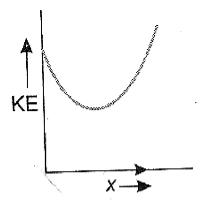
$\text{KE} \propto x^2.$  Thus graph between KE and x will be parabolic.
