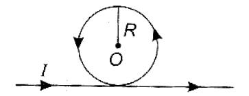
Magnetic field due to long wire at O point
