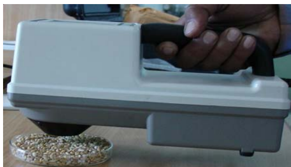
Fig. 2: Measurement of colour of wheat using a colorimeter
