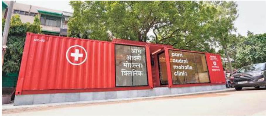
Care on the move: The mohalla clinic at Shakur Basti has been created using shipping containers and can be shifted in trucks from one place to another. •SPECIAL ARRANGEMENT
